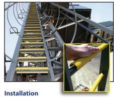
Safeguard® Hi-Traction® Covers are non-load bearing, and are prefabricated for installation over existing surfaces, including steel and composite grating as well as solid metal, wood and concrete. Installation is accomplished using Universal Saddle Clip assemblies, Screws, Bolts and/or Adhesives.
