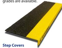
Most slips occur on the leading edge of the stair step, especially when the metal, wood or concrete surface becomes worn or rounded. Water, dust, or oil on the step further accentuates the problem. SAFEGUARD® Hi-Traction® Step Covers are designed to cover the leading edge, providing excellent traction, even in adverse conditions.
